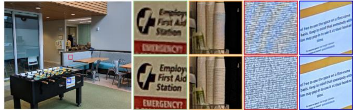
Fig. 1. We present a multi-frame super-resolution algorithm that supplants the need for demosaicing in a camera pipeline by merging a burst of raw images. We show a comparison to a method that merges frames containing the same-color channels together first, and is then followed by demosaicing (top). By contrast, our method (bottom) creates the full RGB directly from a burst of raw images. This burst was captured with a hand-held mobile phone and processed on device. Note in the third (red) inset that the demosaiced result exhibits aliasing (Moiré), while our result takes advantage of this aliasing, which changes on every frame in the burst, to produce a merged result in which the aliasing is gone but the cloth texture becomes visible.
